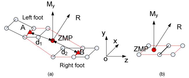
Figure 4. Applying ground reaction forces on ZMP
