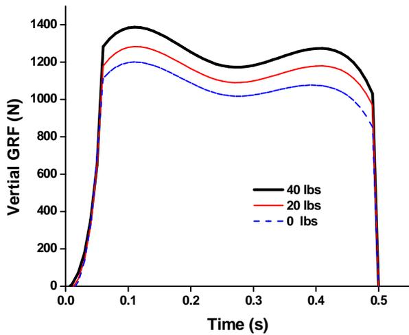
Figure 10. Vertical GRF of walking with backpack
