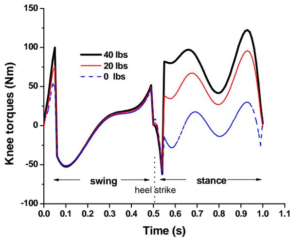
Figure 11. Torque profile of right knee with backpack
