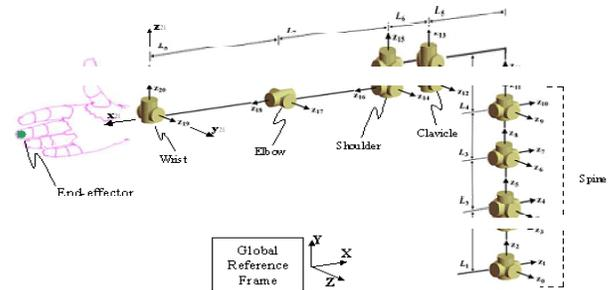
Figure 2: 21-DOF Kinematic Model
