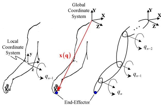
Figure 1: A Kinematic Chain of Joints
