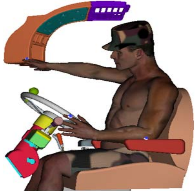
Figure 5. Predicted posture with end-effectors (blue spheres) placed on the multiple locations on the digital human's body, each given its own target (white spheres).
